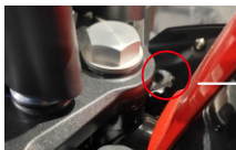
Water tank cover
